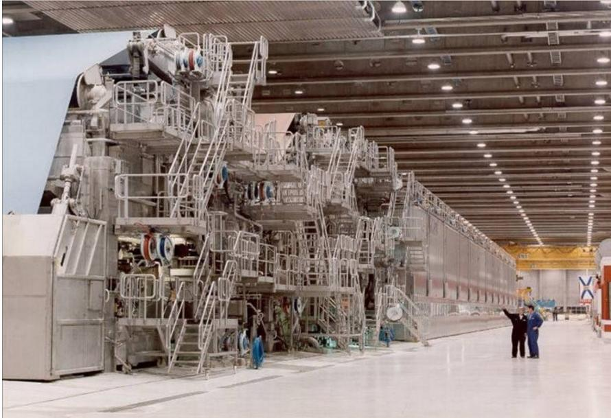
In this case study the customer operates a 20 year old pulp and paper operation in eastern Canada. They are running one of the largest and fastest paper machines on the continent producing coated (shiny) magazine grades of paper.
