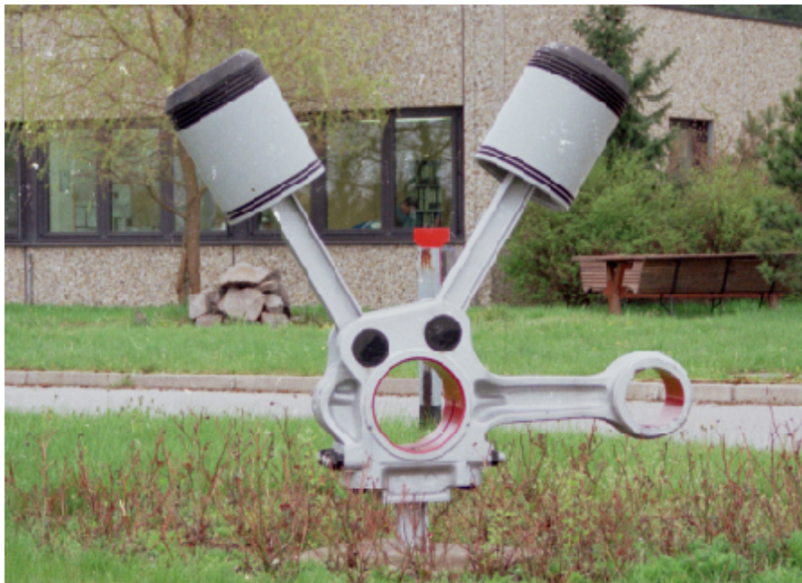
Figure 2. Connecting and articulating rods of an integral-angle gas engine-compressor 2 .
