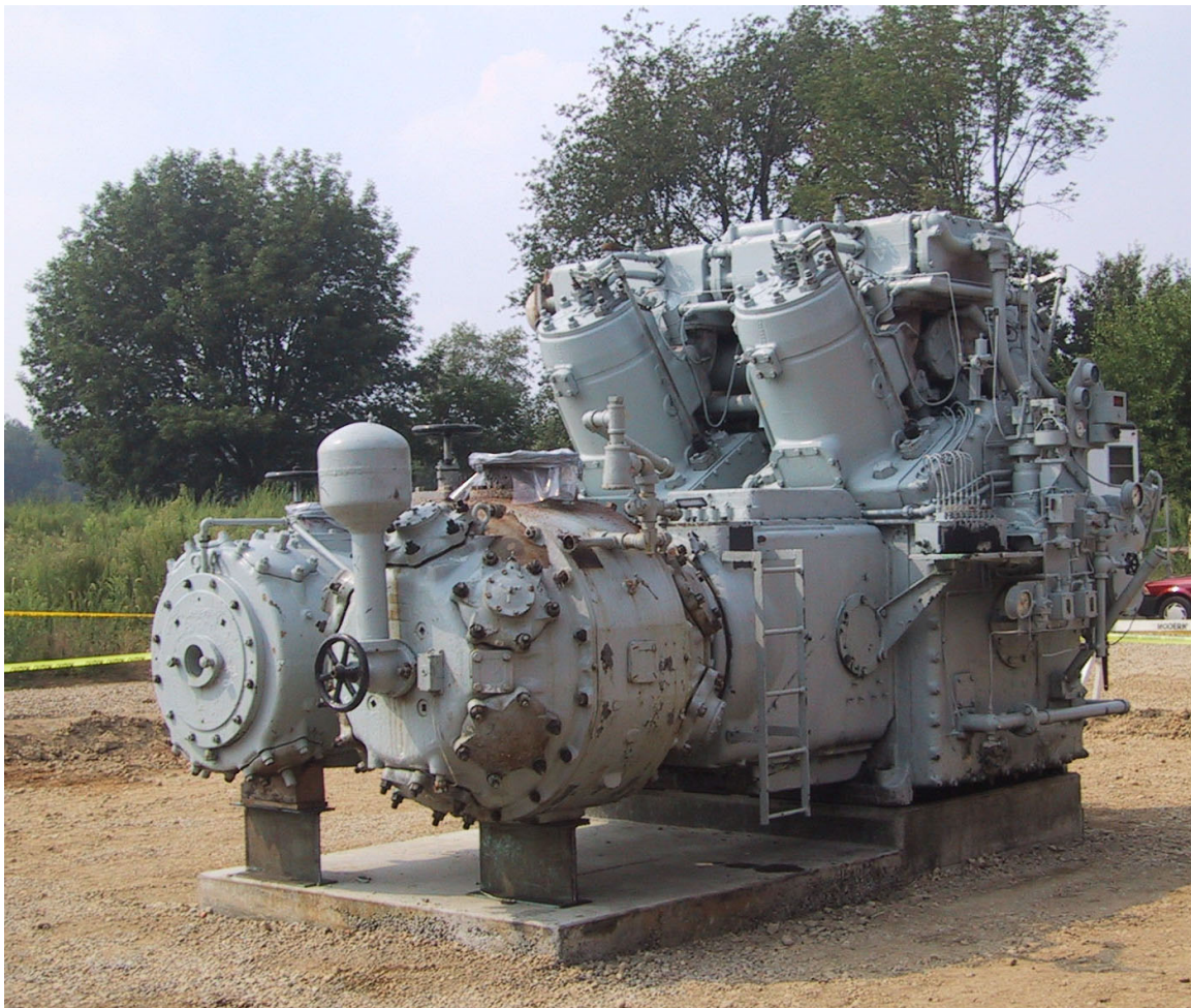
Figure 1. GMV-4 Landmark engine rated at 400 BHP, 300 rpm, 700 ft./min. (3.5 m/s) piston speed. 1
