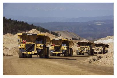
shovel operating at a steady capacity. If you can keep each truck operating even only 10% longer, then each can carry 10% more capacity before replacement. So instead of using 40 trucks to achieve full capacity, if each operates 10% longer, only 36 trucks (10% fewer) are required for the same performance outcome. As each truck costs \$3 - \$5 million (depending on capacity) 4 fewer trucks are needed, for a big saving in capital outlay.
